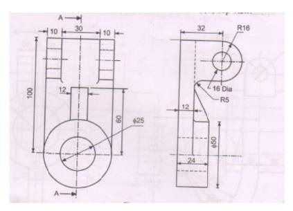
c) Figure shows top view, part auxiliary view and incomplete front view of an object. Draw the given views and complete the front view.
