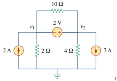
e. Find maximum power in  $R_1 = 4 \Omega$  by using maximum power transfer theorem.
